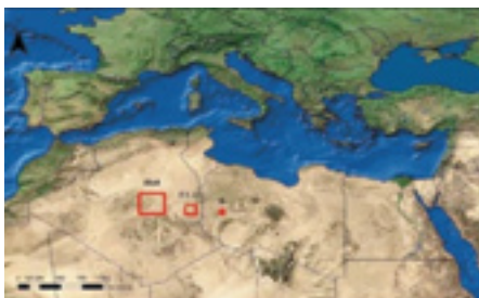
For illustration: Areas of the size as indicated by the red squares would be sufficient for Solar Thermal Power Plants to generate as much electricity as is currently consumed by the World, by Europe (EU-25) and by Germany respectively. (Data provided by the German Aerospace Center (DLR), 2005)
