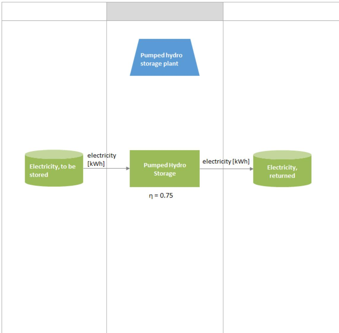
Figure 18: Representation of the pumped hydro storage system.
