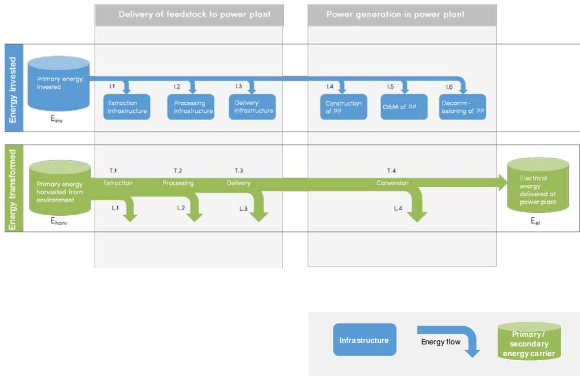
**Figure 1: Energy flows of fuel based power generation system.**
