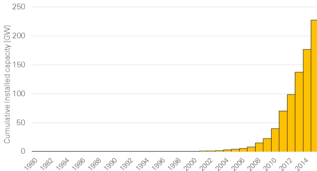
**Figure 38: Cumulative installed capacity of solar PV 1980-2015.**
