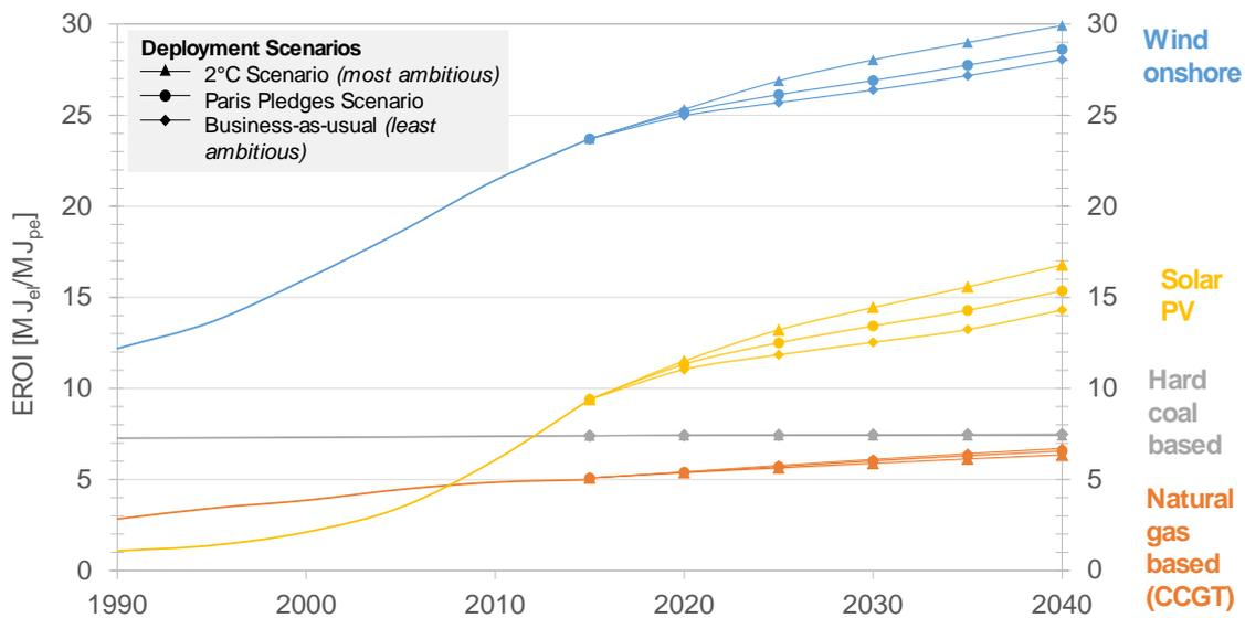
**Figure 43: EROI over time for three alternative deployment scenarios.**
