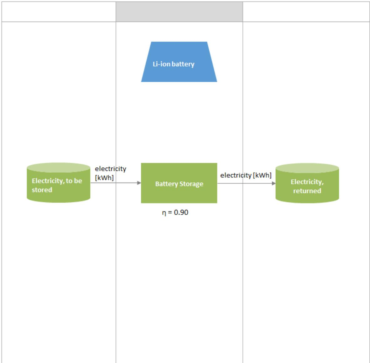
Figure 17: Representation of the lithium-ion battery storage system.
