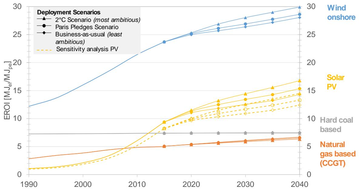
Figure 44: EROI over time for three alternative deployment scenarios, with sensitivity analysis for PV.
