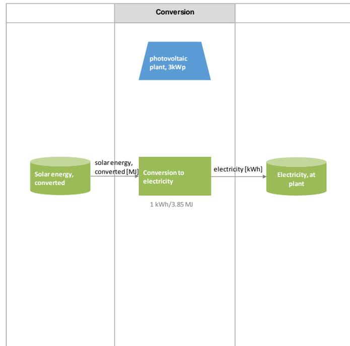
**Figure 12: Representation of the solar PV system in ecoinvent.**
