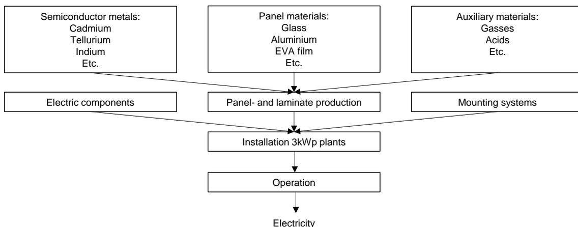
**Figure 11: Components of a cadmium telluride thin film PV system covered by ecoinvent.**
