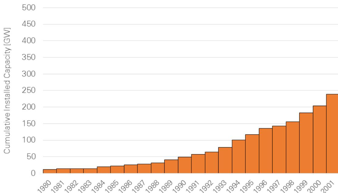
**Figure 31: Cumulative installed capacity of natural gas CCGT 1980-2001.**
