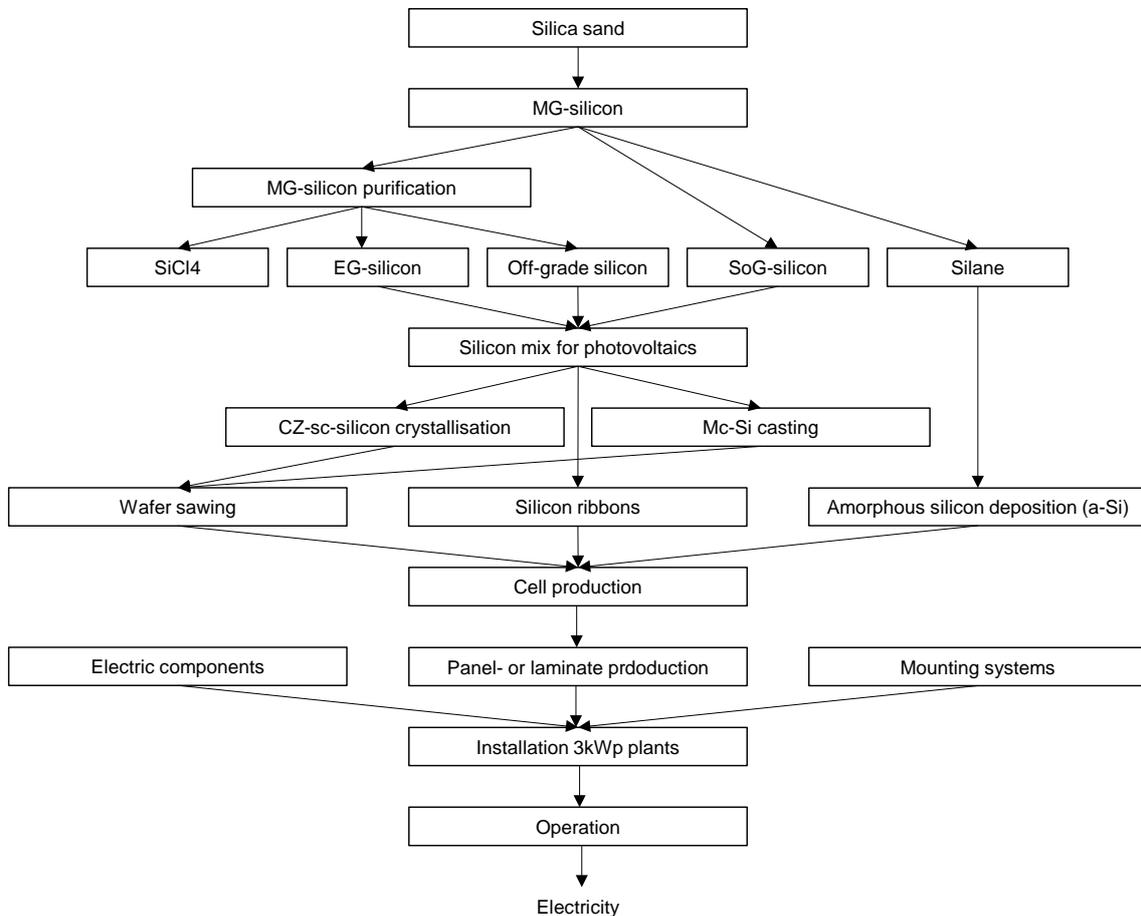
**Figure 10: Components of a crystalline silicon PV system covered by ecoinvent.**
