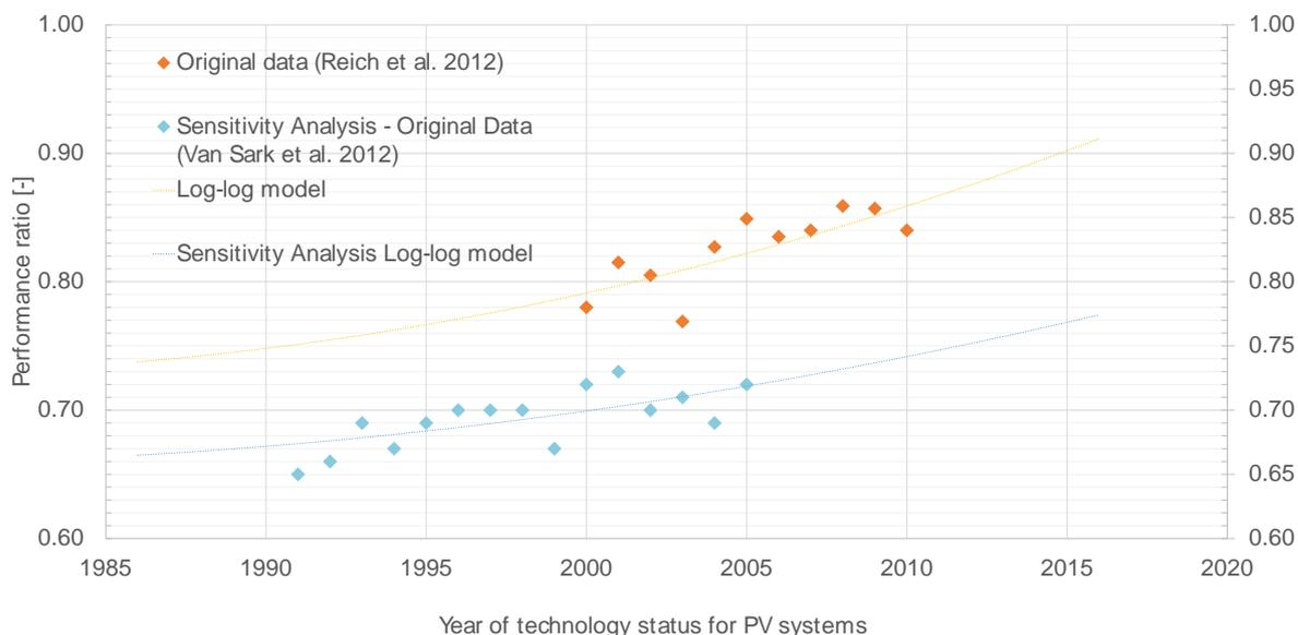
**Figure 40: Performance ratio of PV systems over time (under German climate conditions).**
